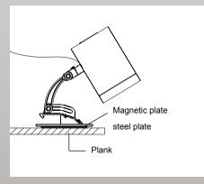
Fixtures can be mounted on steel plate by magnet.
