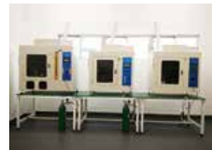
Resistance to heat, fire material test
