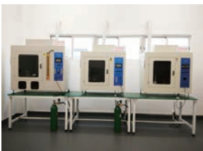
Resistance to heat, fire material test
