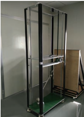
Pendulum impact testing machine
