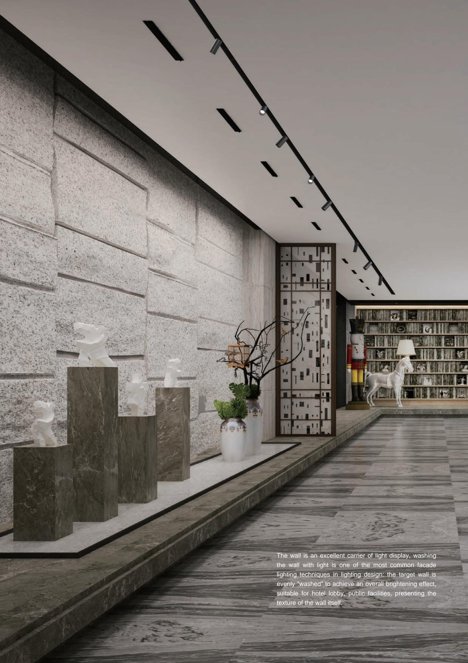
The wall is an excellent carrier of light display, washing the wall with light is one of the most common facade lighting techniques in lighting design: the target wall is evenly "washed" to achieve an overall brightening effect, suitable for hotel lobby, public facilities, presenting the texture of the wall itself.
